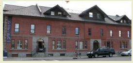
its sandstone quoins, decorated entryways with grey-brick door surrounds, and sandstone keystones; the doorway assemblies were originally detailed with fanlights and wood-paneled reveals. Other Georgian detailing includes the symmetrical façade, sandstone belt course and hipped roofline.
